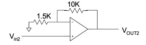
Problem 2 (15 pts) Determine the steady state output for the amplifier shown if the input is  $V_{IN}=3sin(800t+35^{\circ})$ .
